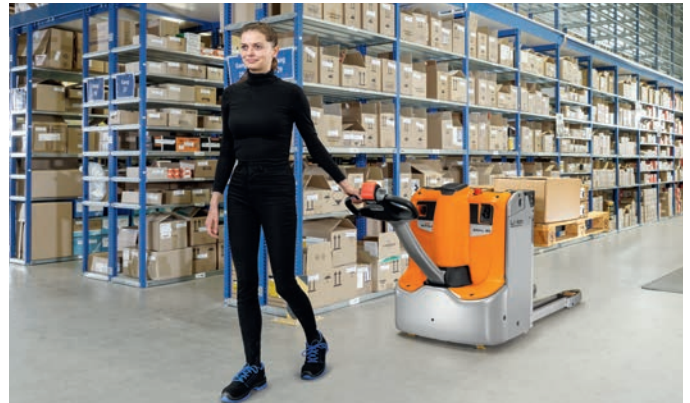
Always safe on the move: thanks to OptiSpeed, the STILL tiller adapts the driving speed continuously to the tiller angle
