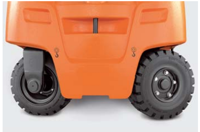
The two tyres can be rotated by 90 degrees to both the left and right.
