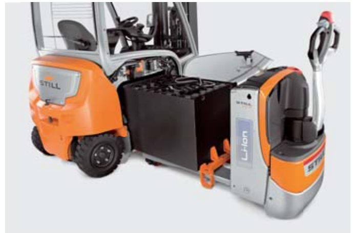
Safe and easy battery change with electric pallet truck.
