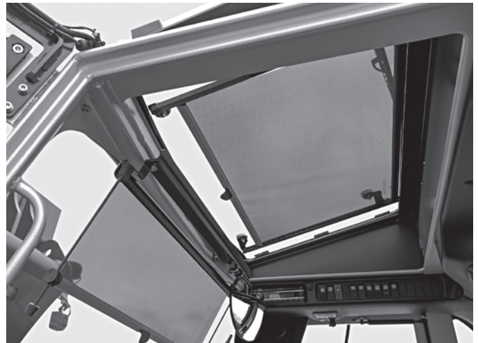
The panoramic armoured glass pane with sun blind provides excellent visibility even on sunny days
