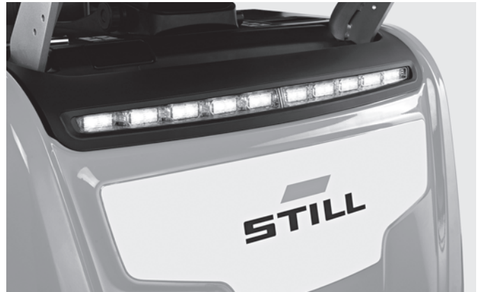
Optional LED daytime running lights for best visibility and improved safety at work 2
