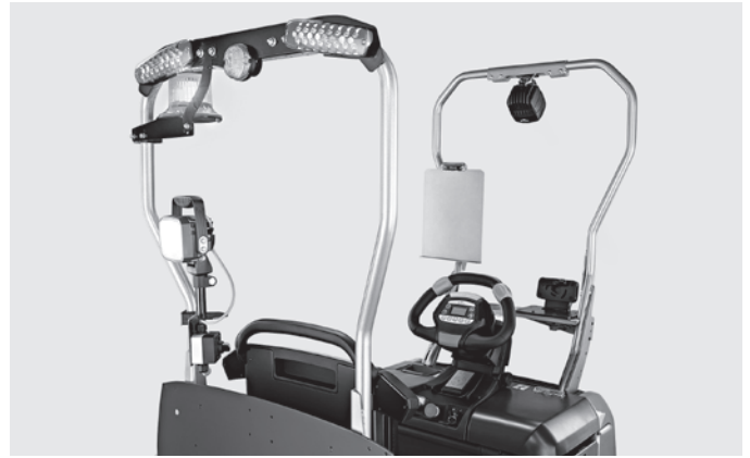
Optional accessory bar for versatile application options and many equipment options including flash lights and working lights 2
