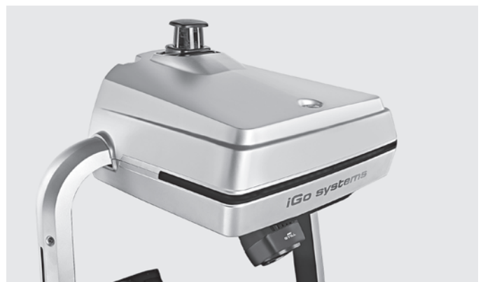
Automatic movement of the LTX 50 iGo systems through the warehouse thanks to the automation box and navigation laser
