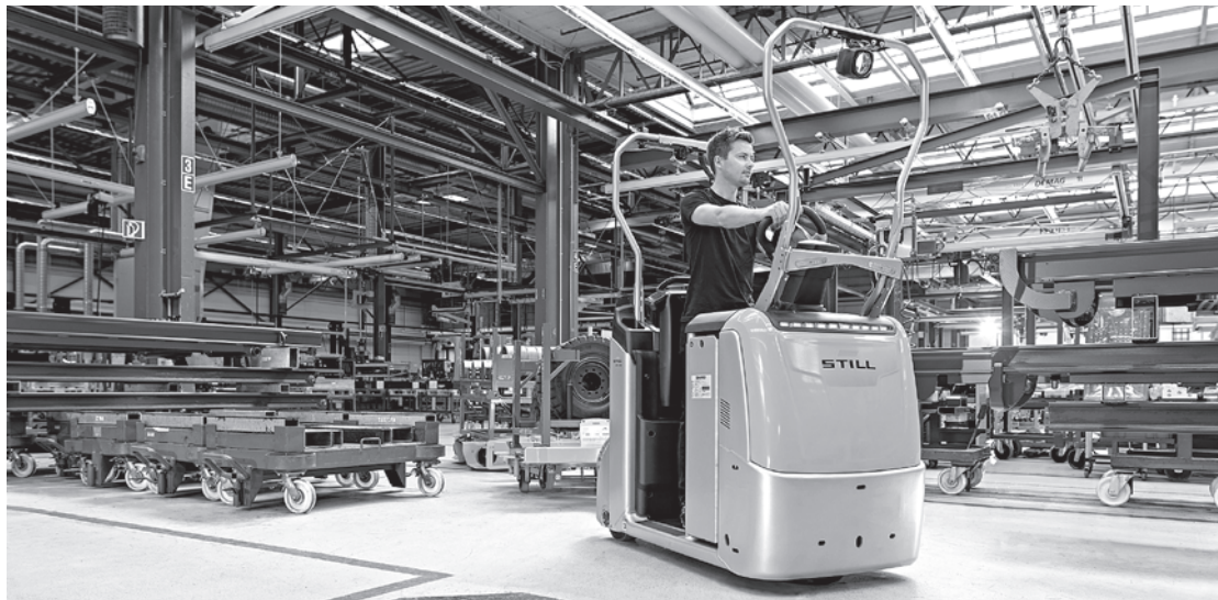
LTX in tugsing train operation
