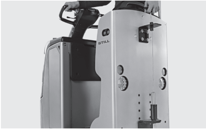
Fast release of coupling from driver's seat 1
