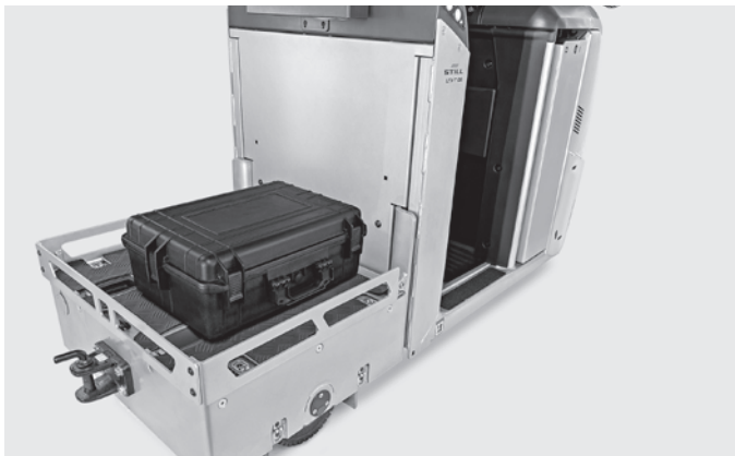
Storage surface with lashing eyelets for up to 600 kg 3
